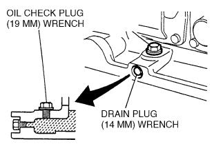
Figure 26. Vibrator Oil Maintenance
